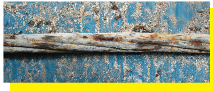
These representative pictures demonstrate the extent of deterioration detected along the transmission line, as displayed in the LF and LMA charts above.
