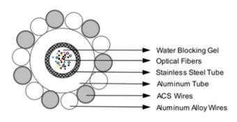
OPGW serves two main systems: power delivery and telecommunications with the following functions: i) protection to overhead lines against lightning strikes and a return path to short circuit currents during system faults, and ii) a high capacity optical communications network.
