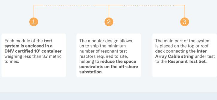
The system can typically be erected in less than two days allowing for one, two or three conductors of a string to be tested in a 10 hour shift. The commissioning tests can be performed during night shifts to ease work planning complications associated with other on-going work on the off-shore substation (OSS).
