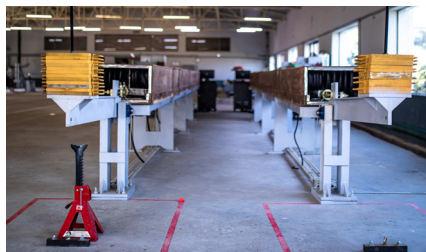
Multi-Purpose Creep Spans
