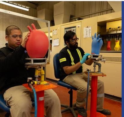
We test rubber gloves to ensure the electrical safety and reliability of PPE used by utility workers in hazardous environments.
