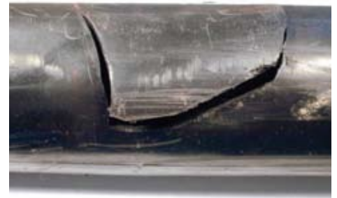
Damaged outer sheath, installed water blocking sub-sheath prevents water ingress
