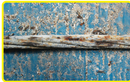
These representative pictures demonstrate the extent of deterioration detected along the transmission line, as displayed in the LF and LMA charts above
