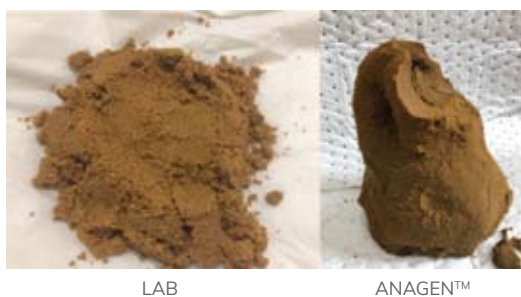
Figure 3. Samples of backfill exposed to (left) conventional LAB based dielectric fluid, and (right) ANAGEN™
