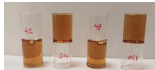
Figure 1. Demonstration of self-healing in exposed ANAGEN™. The sample is exposed to atmosphere and allowed to cure, after which skin strength is demonstrated by inverting the vial.
